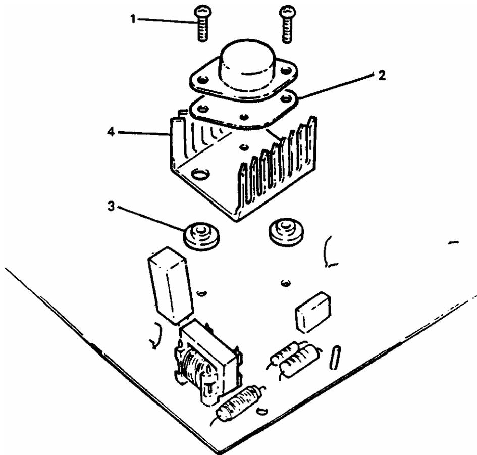
Line Output Transistor (TR202) and SMPSU Output Transistor - Removal/Installation
