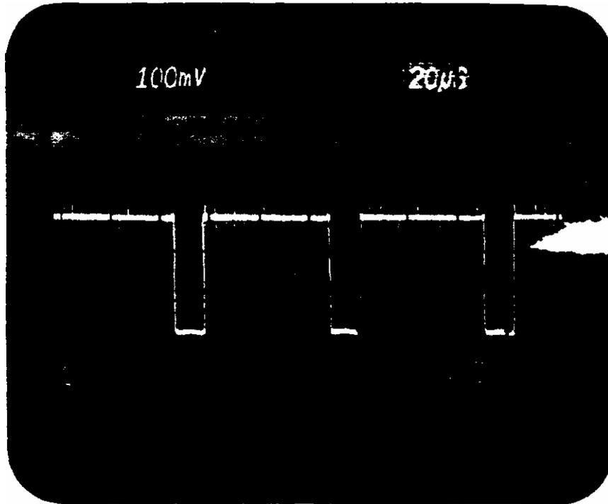
**TR102 COLLECTOR with 10 to 1 scope probe**
