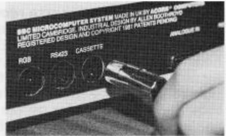
(a) Connecting the cassette recorder to the computer. Note: if three jack plugs are used (as shown), the smallest jack is the remote control for the cassette recorder's motor.
