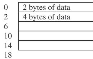
The numbers at the left of the diagram are the addresses in decimal of each field, given as an offset from the location of the start of the block. Each field will hold a particular piece of data. The reference section gives details, for each routine, of what kind of data to put in each field.
