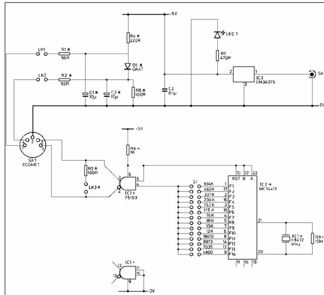
Components marked \* are fitted on terminator boxes.
