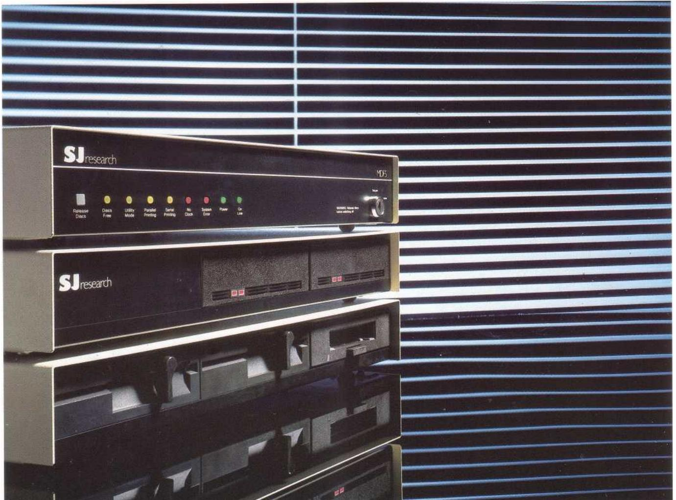
The MDFS is a self-contained modular-disc file server and printer server. The system is capable of supporting a very large network with hard discs and tape backup, but offers a low entry level cost using floppy discs.
